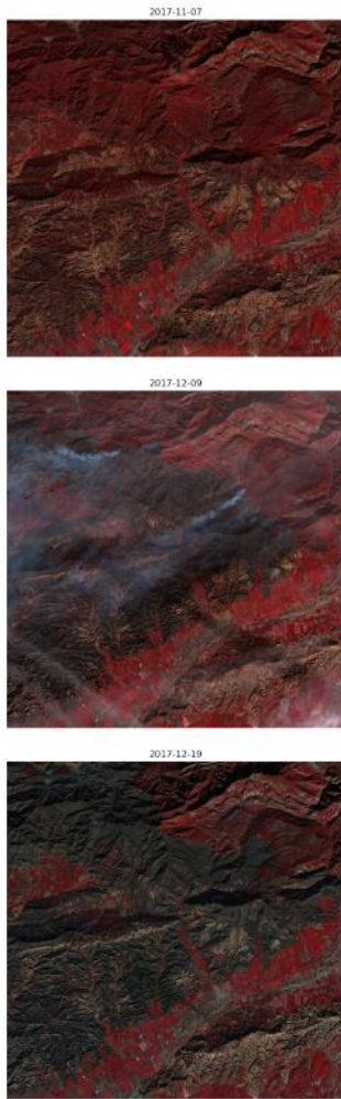
Fig. 1. Sample images capturing the Thomas Fire in California in December 2017. The images show the NDVI on surface reflectance over three Landsat 8 images. The images show the vegetation previous, during and after the wildfire. The second image depicts some smoke, meaning that the wildfire was still being controlled.
